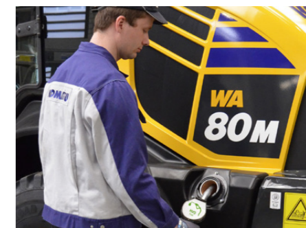
Filling a Komatsu machine with HVO as factory-fill fuel at the KGC plant in Hannover, Germany
