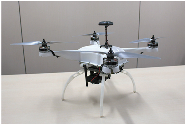
SMARTCONSTRUCTION uses Skycatch-made drone to survey the sites.
