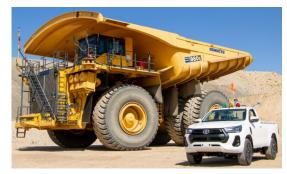
Komatsu autonomous haul truck and Toyota concept ALVKOMATSU\*ALV (Autonomous Light Vehicle)
