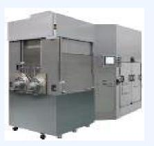
Wire saw for cutting silicon wafers [Komatsu NTC Ltd.]
