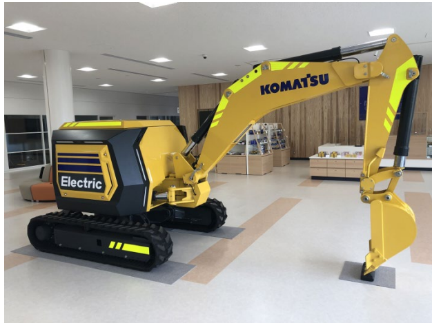
Concept machine for fully electric and remotely controllable mini excavators
