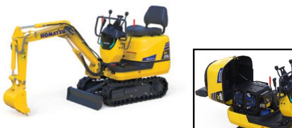
[PC05E-1 electric micro excavator (prototype)]
