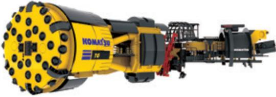
[Mining TBM for underground hard rock mine]
