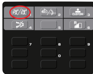
Working mode selector switch
