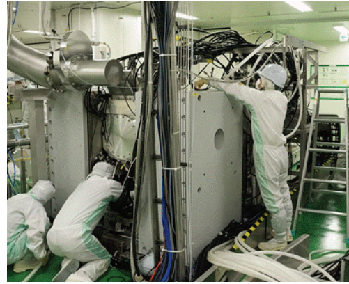
図 12 Picture of proto-type EUV source GL200E
