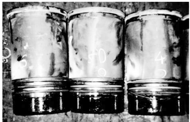
Photo 7 Result of field test of non-amine type coolant
