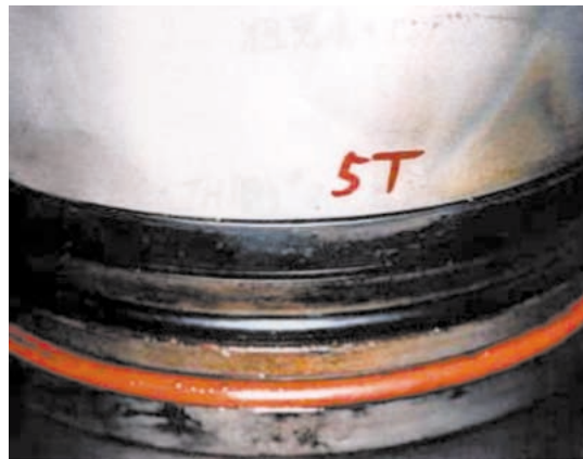
b) Acceptable as no cavitation is noticed on seal
