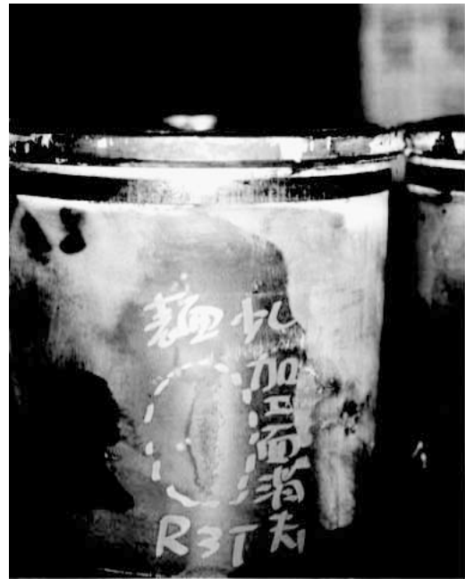
Photo 3 Result of engine bench test for non-amine type coolant (cylinder liner cavitation pitching at initial stage of development)
