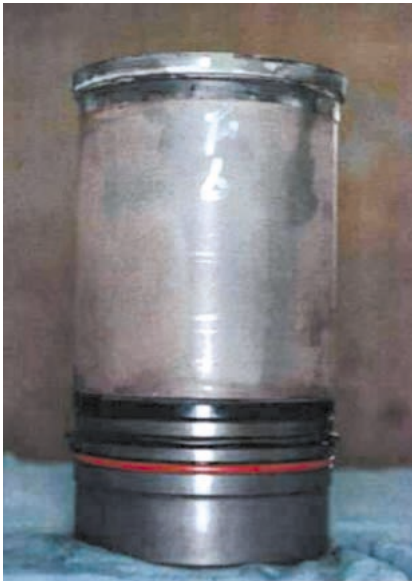
a) Acceptable as no cavitation pitching, rust, etc. are noticed on cylinder liner surface.
