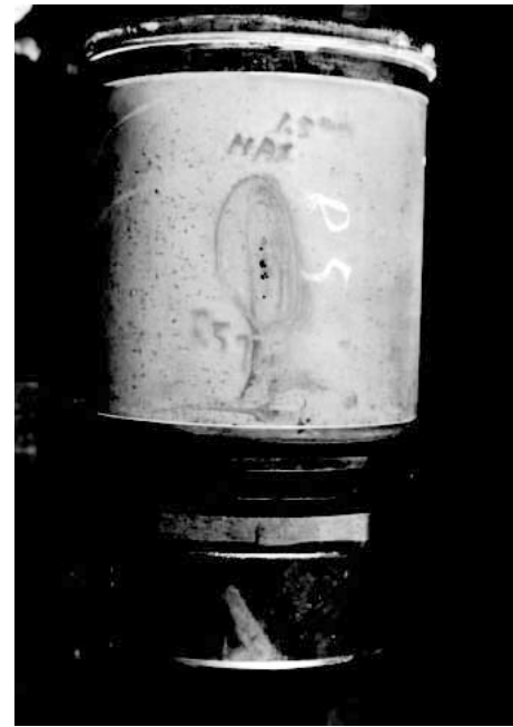
Photo 1 Example of using commercially available coolant (at 500 h in engine bench test)
