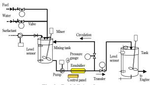
Fig. 3 Fuel Mixing System
