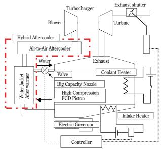
Fig. 7 Engine System
