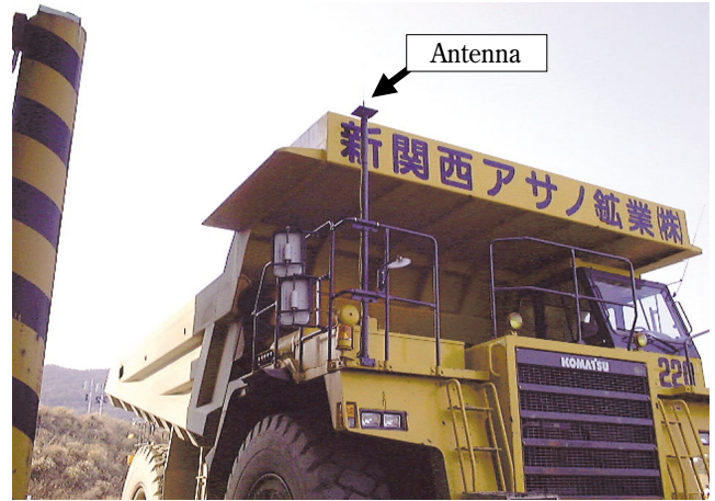
Photo 1 Satellite communication equipment mounted on vehicle
