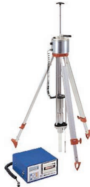
Fig. 5 Appearance of Caspol – simple soil bearing – force measuring instrument
