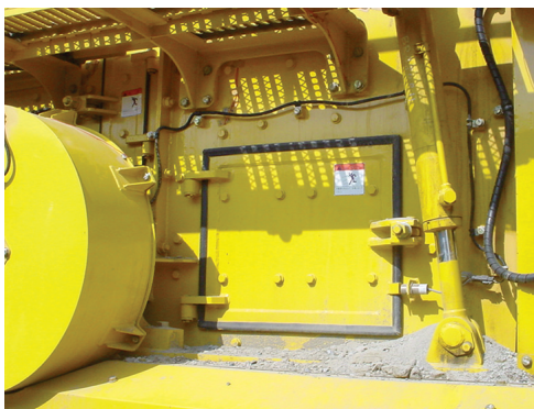
Photo 3 Large inspection window
