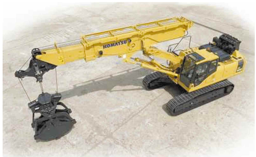
Photo 1 Appearance of the PX500 low-profile, great-depth clamshell
