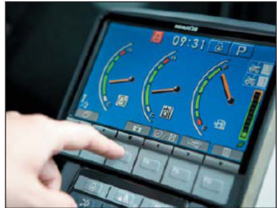
Fig. 15 Large multi-monitor display (VHMS embedded)
