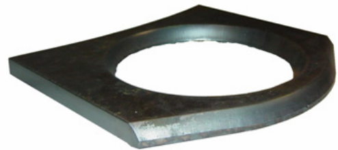
Fig. 10b Sample of machined groove Plate thickness 19 mm, groove angle 35°, root height 5 mm.
