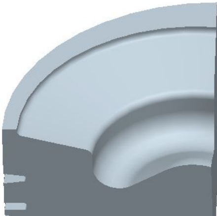
Fig. 5 Shape of combustion chamber for SAA4D95LE-5 engine
