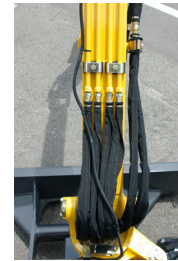
Cover to prevent splashing of pressurized oil
