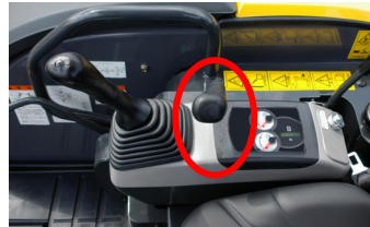
Change in installed position of automatic travel transmission switch
