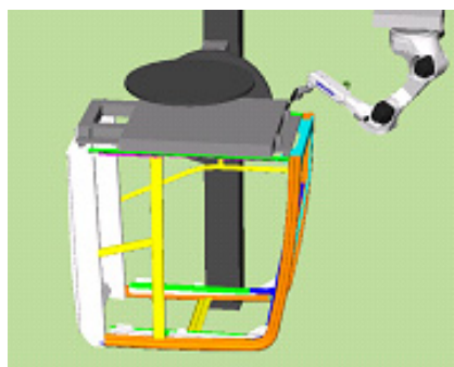
Fig. 21 Welding on floor side
