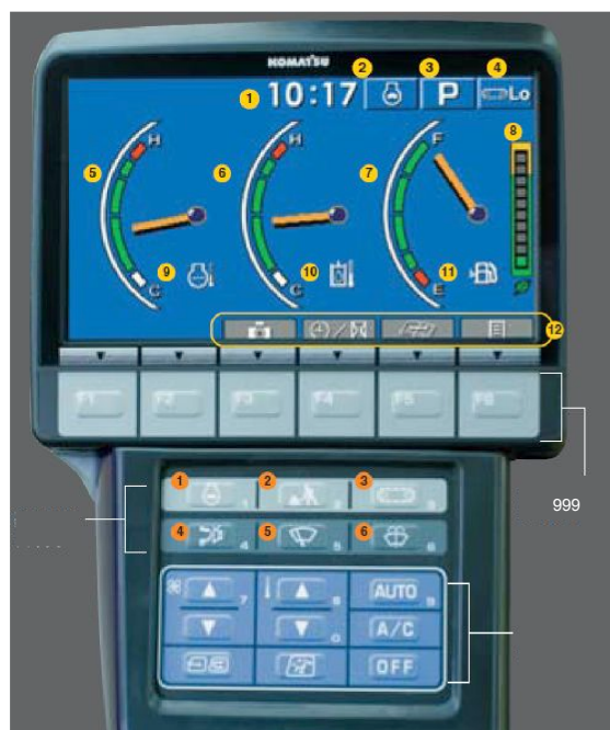
Fig. 15 New large-sized color multi monitor and function switches (Extract from PC228US-8 Catalogue)
