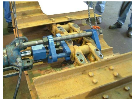
(1) The shoe plate is dismantled and a special jig is mounted.
