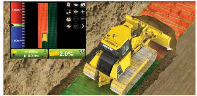
Fig. 3 Intelligent Machine Control bulldozers 3-D construction data
