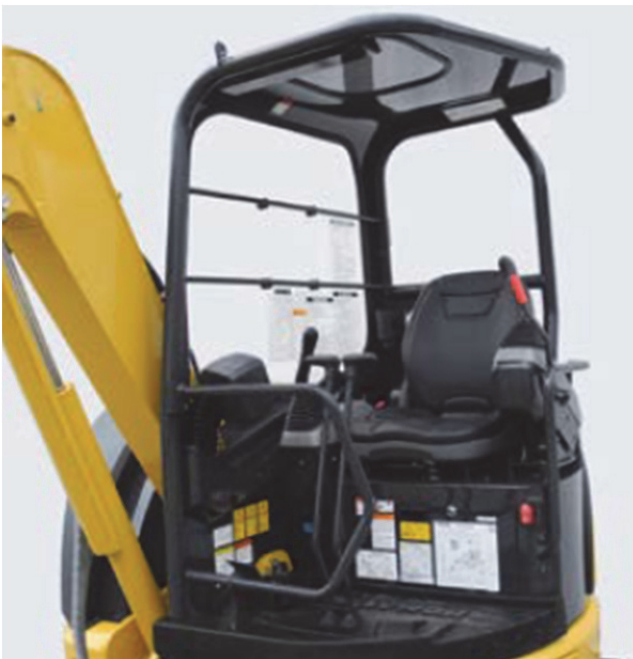
Fig. 3 TOPS canopy (from company data)
