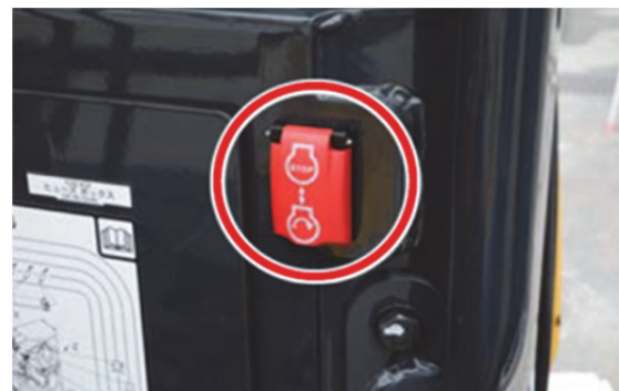
Fig. 6 Secondary engine stop switch (from company data)
