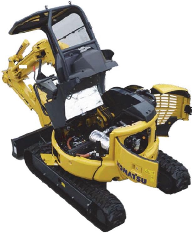
Fig. 9 Floor tilt-up mechanism and full opening cover (from company data)
