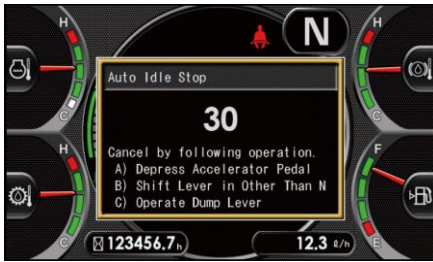
Fig. 3 Introduction of auto idle stop count down
