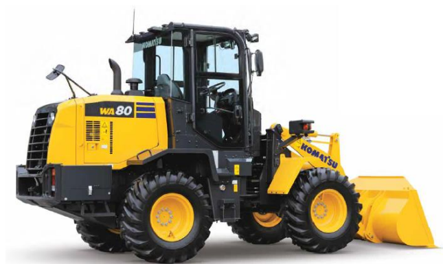
Fig. 1 WA80-8 (from the photograph in the catalog)
