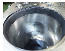
Fig. 12 Appearance of the inner surface of the cylinder
