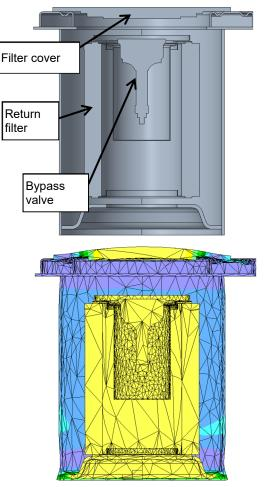
Fig. 6 Deformation of the filter case by pressure
