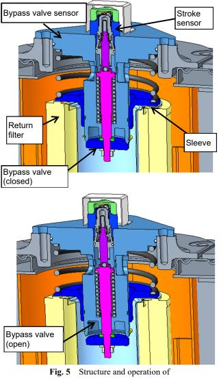
the Komatsu bypass valve sensor
