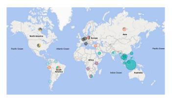
Fig. 8 Monitoring filter conditions of machines all over the world through KOMTRAX
