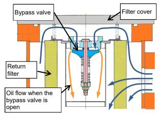
Fig.3 Structure of the bypass valve
