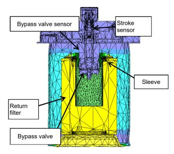
Fig. 7 Deformation of bypass valve sensor by pressure
