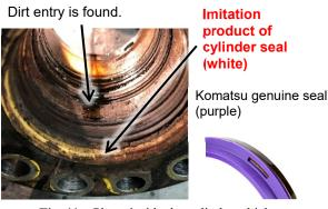
Fig. 11 Photo inside the cylinder which uses an imitation product
