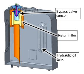
Fig. 2 Return filter and bypass valve sensor in a hydraulic oil tank
