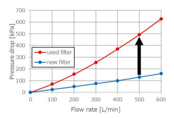
Fig. 10 Pressure loss of filters collected for investigation
