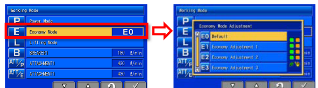
Fig. 9 Easier adjustment of the work mode
