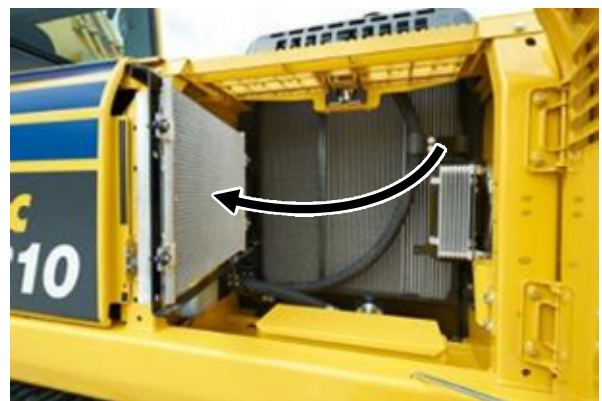
Fig. 12 Swing type air conditioner condenser (PC210-10M0 only)
