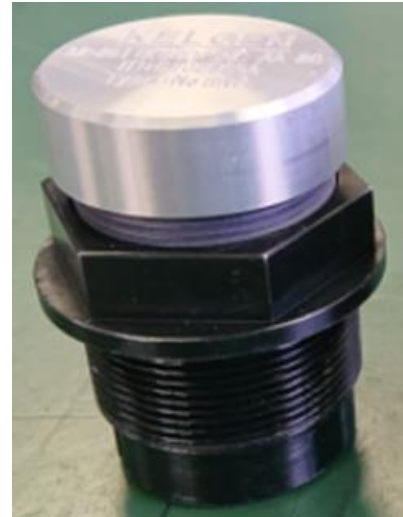
Fig. 8 Oil contamination concentration sensor
