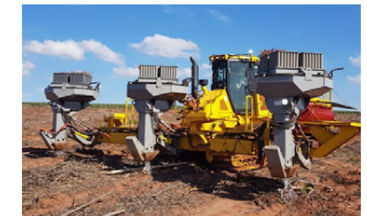
Crawler planter equipped with Bracke-made attachments on Komatsu-made bulldozer
