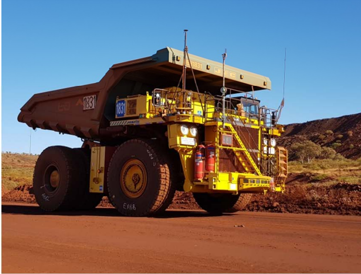
A standard truck 830E with the AHS retrofit kit running in autonomous mode at Rio Tinto's mine in Australia
