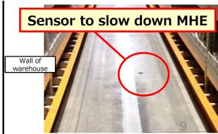
➤ When 2<sup>nd</sup> forklift enters, sensor works and reduce speed automatically.
