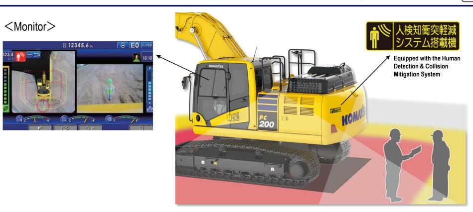
When starting to travel or even while traveling at low speed, the excavator stops low-speed traveling as soon as person(s) is detected inside the stop-controlled area.
