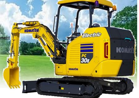
Output (net): 17.4kW Standard bucket capacity: 0.09m<sup>3</sup>
