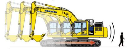
When starting to swing from the halting position, the excavator stops swinging as soon as it detects person(s) inside the stop-controlled area.
