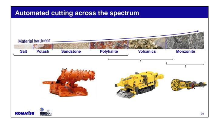
We now have continuous cutting methods for a variety of applications across all types of material hardness. Our proven continuous mining solutions can be used to help operators reliably cut through materials from the softest -- like coal, salt and potash -- to volcanics and some monzonite applications.
