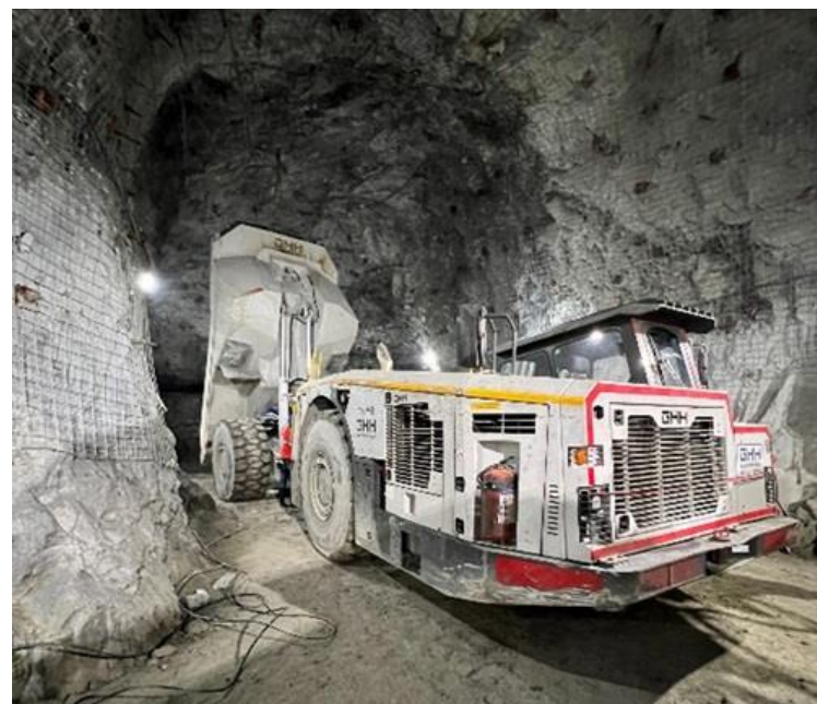
GHH-made MK-42 underground dump truck
