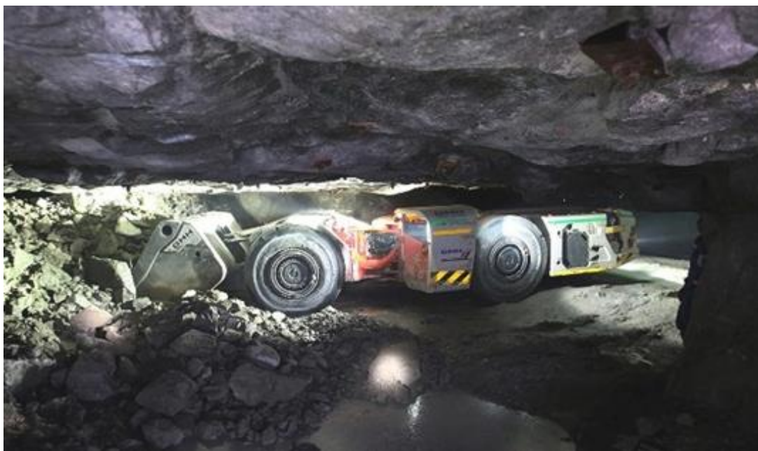
GHH-made LHD (Load Haul Dump) designed for use in narrow veins
