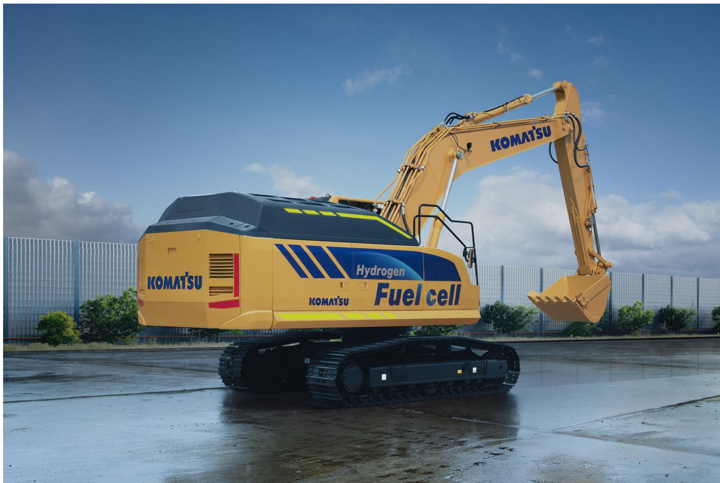
Concept machine for a medium-sized hydraulic excavator equipped with a hydrogen fuel cell.
