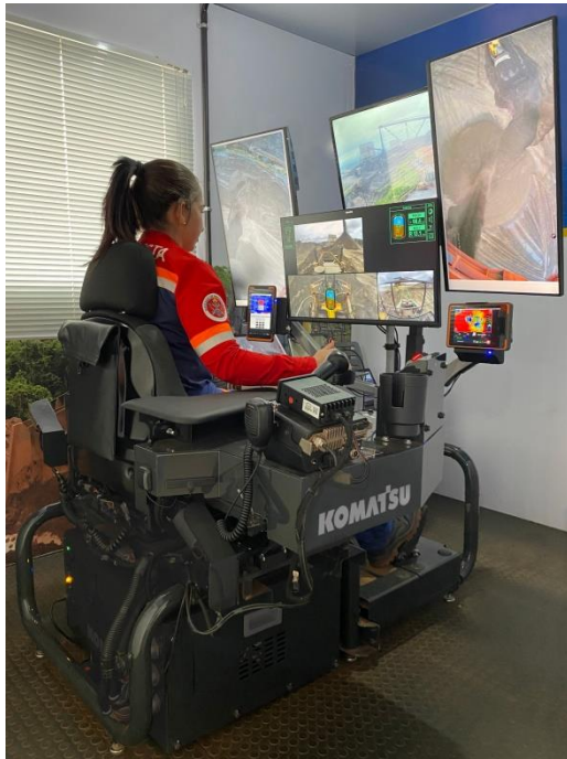
Bulldozer D375Ai-8 operating remotely at Minas-Rio iron ore mine in Brazil.
