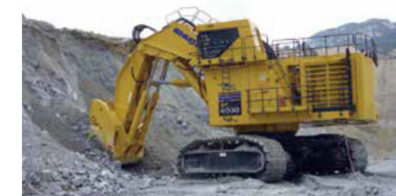
PC4000 mining shovel (bucket capacity: 22 cu. meters or 29 cu. yards)
