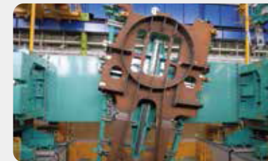
溶接ポジショナー（大型建機用） Welding positioner (for large construction equipment)
