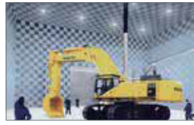
大型音響実験室での騒音計測 Noise Measurement in the Largest-Scale Acoustic Testing Laboratory
