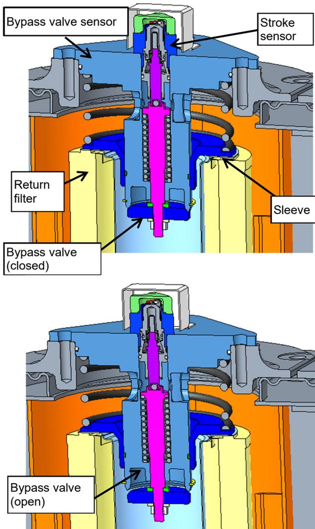
Fig. 5 Structure and operation of the Komatsu bypass valve sensor
