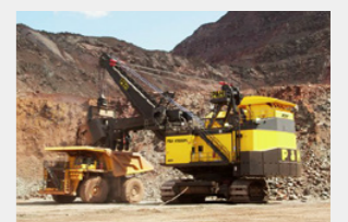
Komatsu Mining Corp. rope shovel and Komatsu super-large dump truck
