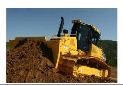
D61PXi-23 medium-sized bulldozer which features the world's first\* full automatic blade control
