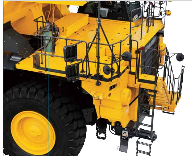
Grease pump and reservoir
