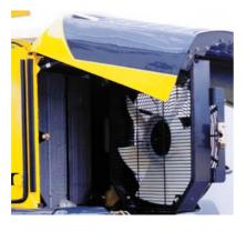
air-to-air cooler and oil cooler are mounted side-by-side for more efficient cooling and easy cleaning. A fully-opening, gas spring assisted rear grill gives the operator excellent access to the swing-out fan and coolers.
