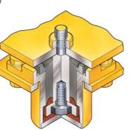
with rubber cushions, and the cab sealing is improved to provide a quiet, low-vibration, and comfortable operating environment. Pressurization in the cab keeps dirt out further enhancing the operator's comfort.
