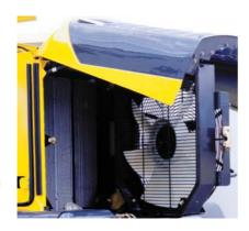
air-to-air cooler and oil cooler are mounted side-by-side for more efficient cooling and easy cleaning. A fully-opening, gas spring assisted rear grill gives the operator excellent access to the swing-out fan and coolers.
