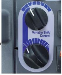
operator to adjust his machine speed in confined v-loading applications. When in 1, the operator can adjust his travel speed using the variable shift switch to match his machine speed and hydraulics to the distance he must travel.
