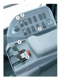
1:Cut-off ON/OFF switch 2:Cut-off adjustment switch 3:Fan reverse ON/OFF switch 4:Boom control 5:Bucket control
